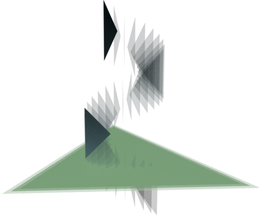
Figure 2: Test problem: CCD of a triangle moving rigidly along a screw trajectory, and another deforming triangle. The triangle on top rotates and moves along an axis until the two primitives come into contact.
